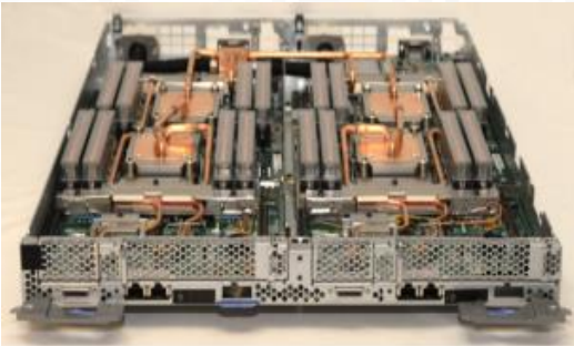
2013: NextScale nx360M5 WCT 45°C-50°C; 约85%的热回收 100% w/ RDHx @ 25°C
